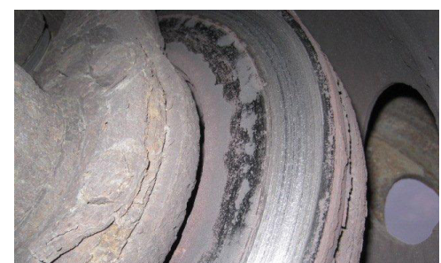
Metal-to-metal contact. OOSC, Part II, a.(6)(c) / 393.48(a)-U.S.
