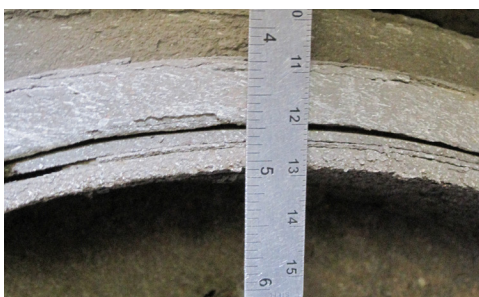
Worn out linings. OOSC, Part II, a.(5)(c)vii / 393.47(d)(2)-U.S.
