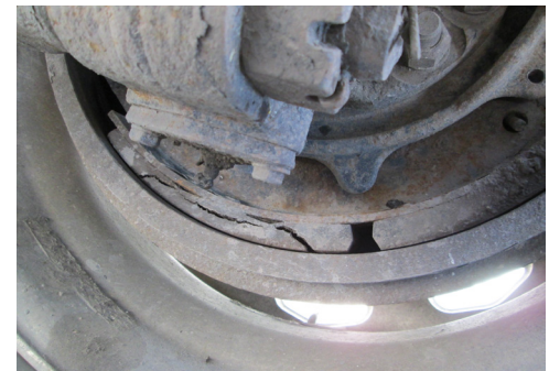
Cracked lining. OOSC, Part II, a.(5)(c)iii / 393.47(a)-U.S.
